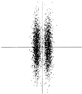
Fig. 9. An illustration of projection pursuit and the “interestingness” of non-Gaussian projections. The data in this figure is clearly divided into two clusters. However, the principal component, i.e. the direction of maximum variance, would be vertical, providing no separation between the clusters. In contrast, the strongly non-Gaussian projection pursuit direction is horizontal, providing optimal separation of the clusters.
