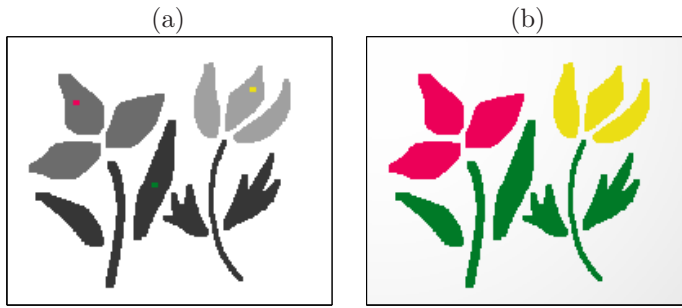
Figure 4: (a) The given grayscale image with small regions with color. (b) The colorization result using the proposed method ( r = 0 , p = 2 , \sigma_1 = 0.001 , and \sigma_2 = 10 ). Notice that only one dab of color is given for each four different colors, and all the regions are colorized according to the intensity similarity.
