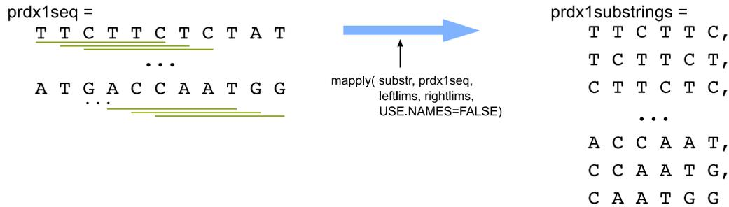
Figure 2: Dissecting a large sequence into a vector of overlapping fragments using the function 'mapply'.
